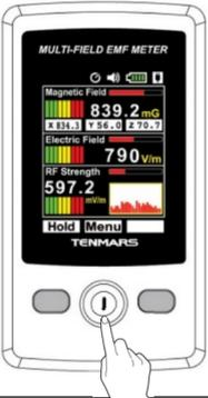
In the measurement mode, press the middle button to enter the main menu
